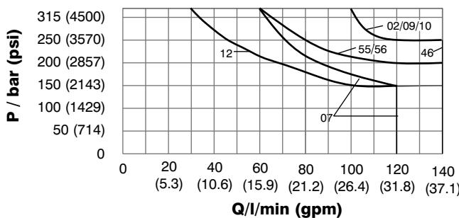
This functional limits have been obtained with warm solenoid condition and at 10 undervoltage from the selected nominal value. All flow data given is considered for 2 flow directions (eg. P to A and simultaneously from B to T). For single flow direction only (4-Way-Valve used as a 3-Way-Valve) the permissible flow must be reduced by as much as 25....30 in comparison to the data shown.
