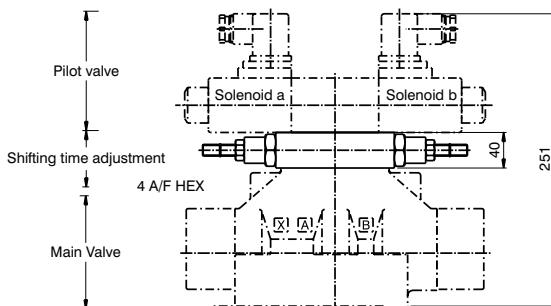
The shifting time adjustment is affected by a double throttle valve with check, which is mounted between main and pilot valve. The illustration depicts the "meter out" control. For "meter in" invert the control.
